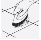
STEP 3. Scrub the surface to release any residues. Machines can be used.
