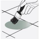
Spread out evenly using a paint brush and leave for 30 - 40 minutes
