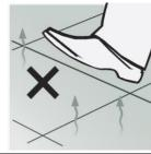
STEP 5. Allow surfaces to completely dry before sealing or allowing traffic.
